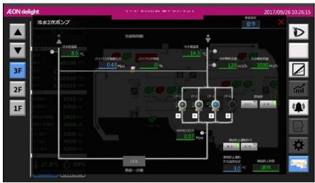
Remote surveillance and automatic control of a climate control system for large-scale commercial facilities by the open network system
